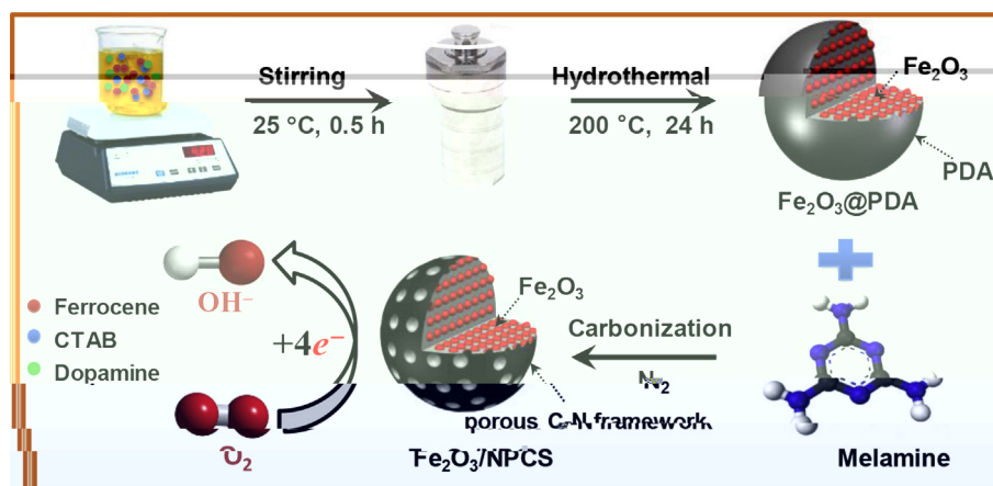
Scheme 2 e Schematic diagram of the reaction process for synthesizing \text{Fe}_2\text{O}_3/\text{NPCS} .
